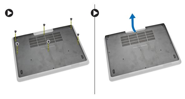
**NOTE:** You may need a sharp tool to pry the base cover from its edge.
