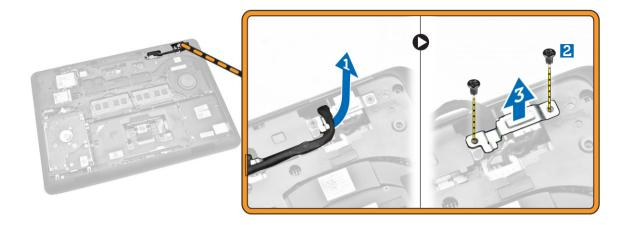
**4.** Disconnect the power-connector port cable from its connector [1] and remove the power-connector port from the computer [2].
