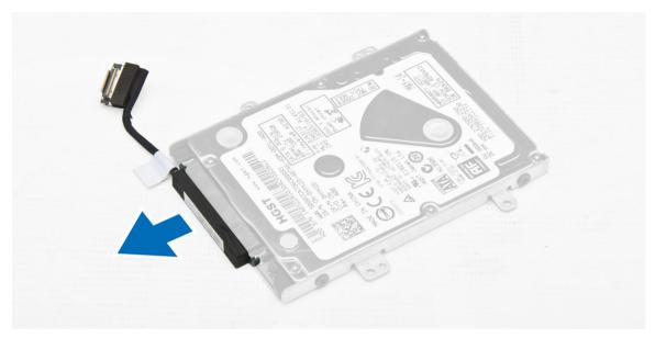
**6.** Remove the screws that secure the hard-drive bracket to the hard drive [1] and remove the hard drive from the hard-drive bracket [2].
