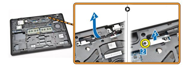
**5.** Disconnect the display cable from its connector [1] and release the display cable [2].
