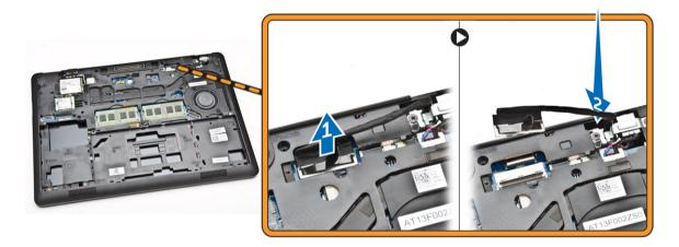
**6.** Remove the screws that secure the display assembly [1] and lift the display assembly to remove it from the computer [2].
