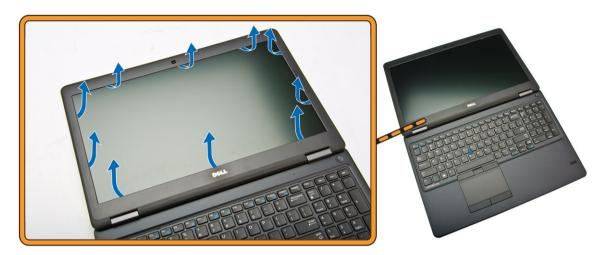
**3.** Remove the display bezel from the display assembly.
