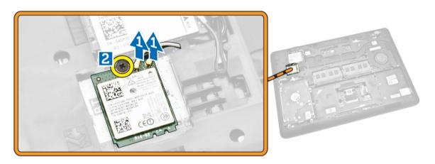
**4.** Remove the WLAN card from the computer.
