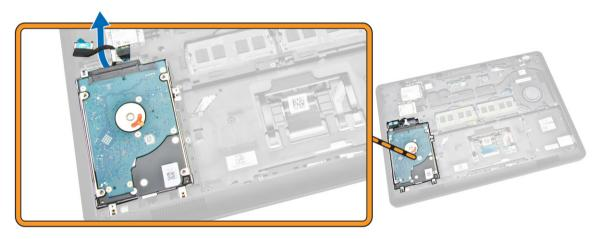
**5.** Pull to release the hard-drive cable from its connector.
