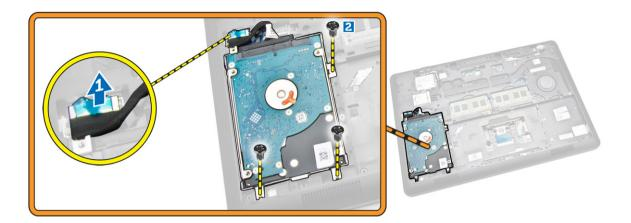
**4.** Remove the hard-drive assembly from the computer.
