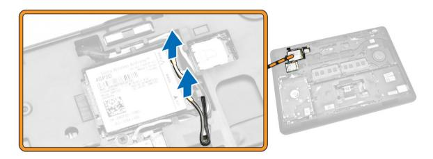
**4.** Remove the screw that secures the WWAN card [1] and remove the WWAN card from the computer [2].
