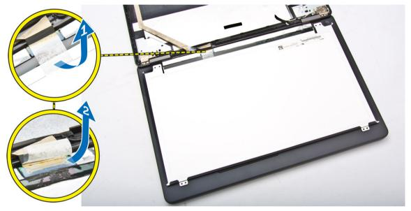
**5.** Disconnect the eDP cable from its connector [1] and remove the display panel from the display assembly [2].
